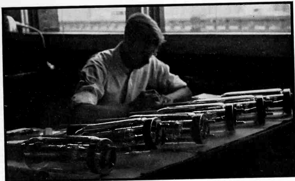
Experimental tube shop; Checking watercooled power tubes
