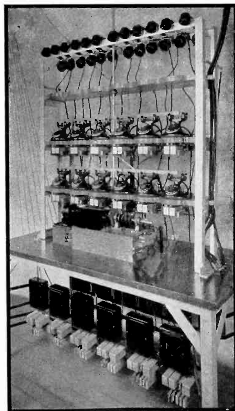
Fatigue testing: This machine operates the contacts in handset mountings, under conditions simulating actual use
