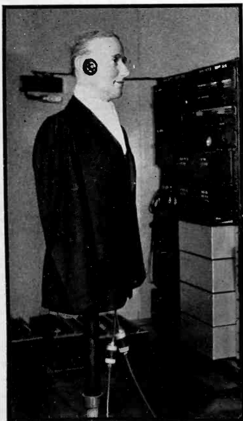
Oscar: Telephone transmitters as ears tell what a human would hear in Oscar's place. He is an important laboratory assistant
