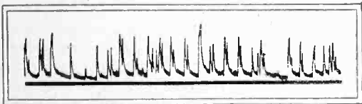
Fig. 1. Oscillogram of commutator roughness
