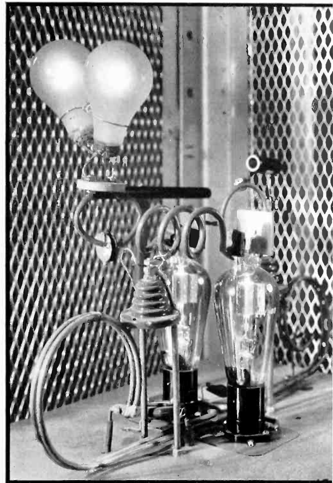
Life test: 304-A's in a fifteen-meter oscillator of unusual designs
